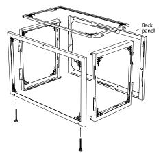
**2.** All panels fit together with a numbered tab and slot system.
