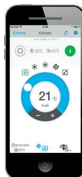
**Control** the operation mode, set temperature, air purification, air flow rate and direction
